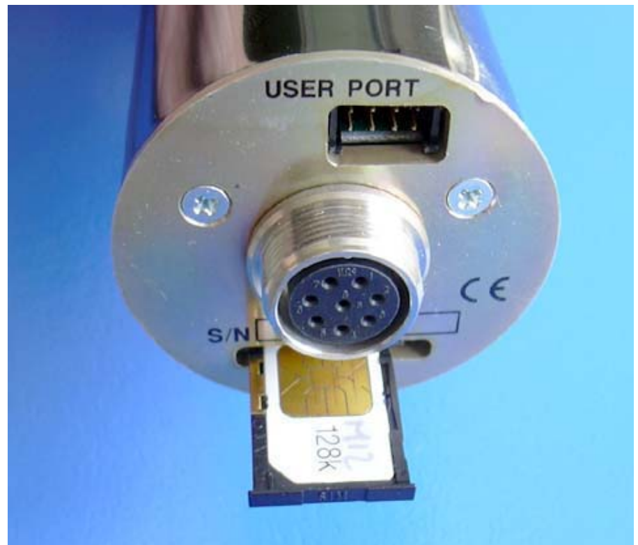
Fig. 3-1 SIM card installation
